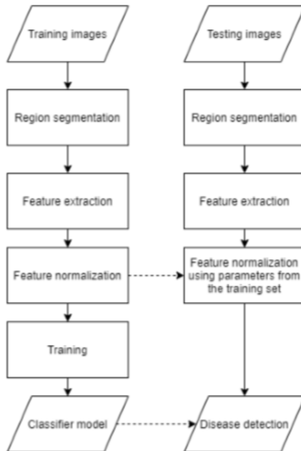
Figure 2: Flowchart of the basic training and testing steps
